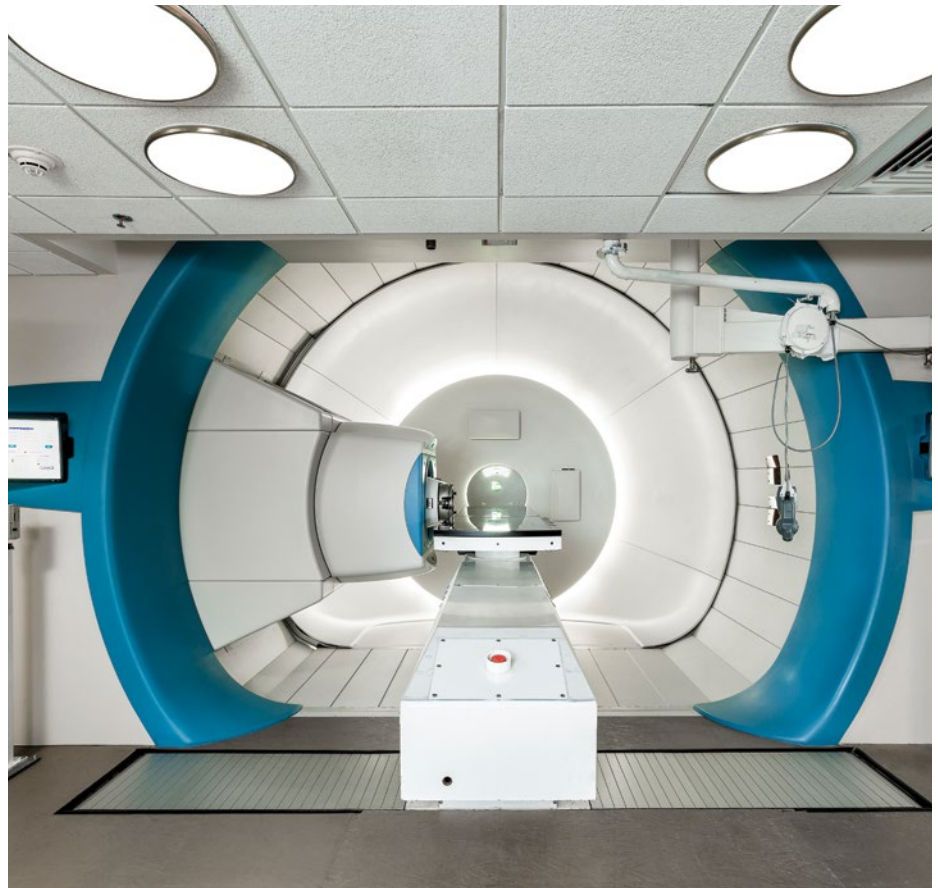
Proton therapy is delivered while you lie on the treatment table. A gantry rotates to deliver therapy precisely to the tumor site. Photo credit: Ryan Ketterman.
